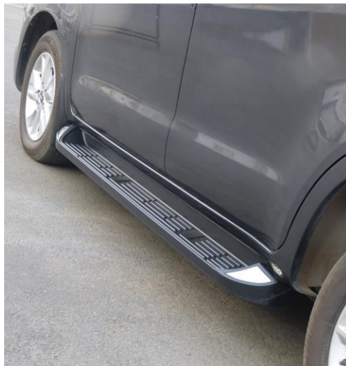
Goldsun footstep using Absolac E502 BML (image courtesy of Goldsun)
